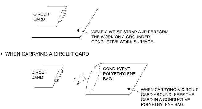
The mark shown below is attached to the sheet for the work in which circuit cards are handled. When engaging in such work, the installer must be careful not to cause damage by static electricity.
